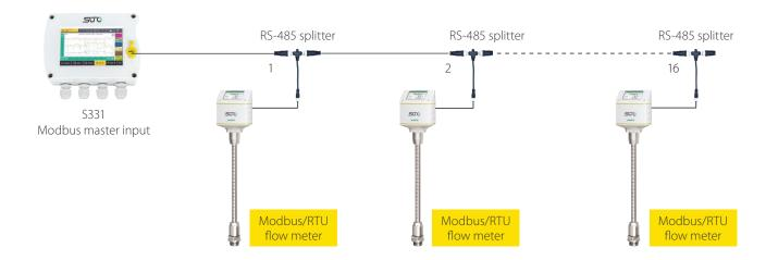
Flow meters can be easily integrated into a Modbus/RTU network (daisy chain)
