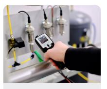
Detection at medium distance for locating the leakage area.
